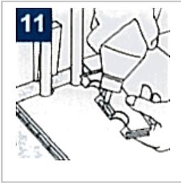
Apply P.V.A. adhesive to the edges of the cut board and fit into place. Care should be taken to leave an expansion gap between the board and the wall.
