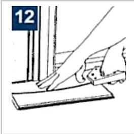
Door frames and other wooden elements should be sawn off to allow the board to slide underneath.
