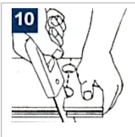
Cut the board at an angle of 45°.
