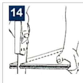
To calculate the exact width of the last board, lay the board over the last but one line of boards (tongue facing the wall). Place another board face down over the board to be cut, remembering to leave the expansion gap, mark the board to be cut.
