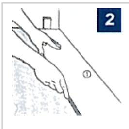
Lay out the first board ensuring the groove is towards the wall. Place a wedge between the end of the boards and the wall, this will ensure that you have an expansion gap (minimum 12mm). Complete the first line of the boards, do not glue the boards at this stage.
